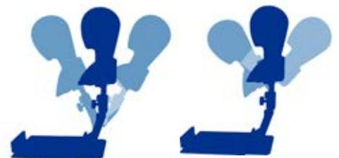
The HSM IV can be bent, turned, and adjusted in various heights.
